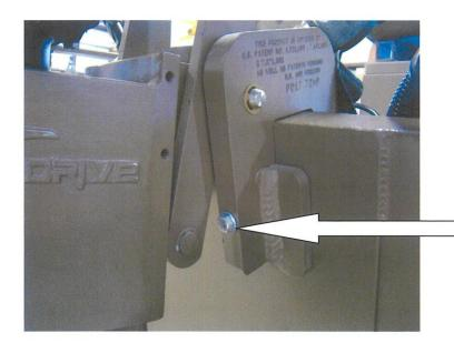
Located on the back of the transom bracket there are three sets of holes on each side. Drill a 3/8" hole through the transom. One on each side in the holes on the bracket. Use the 3/8" bolts and nuts supplied with your unit to secure the bracket in the holes drilled.
