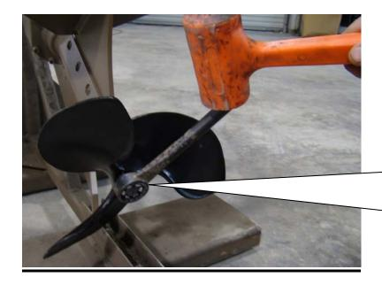
Using your 1-1/8" wrench tighten the prop. Next lightly tap the wrench to further tighten the nut to align the prop shaft hole with one of the slots in the nut. Install cotter pin.
