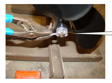
Remove the cotter pin from the prop shaft.
