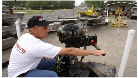
Step 2. Pull the reverse release pin down. Pull the tiller toward you slightly, then release the pin and continue pulling the tiller toward you until you here the unit click. (Once you release the pin you will not have to pull the pin again until you are ready to go back into the forward position.) Push the tiller handle away from you again like in step 1 and repeat. When your reverse clicks for the fourth time your pin will locate in the reversed locked position.
