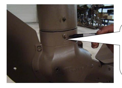
YOUR LOWER UNIT TOP BEARING IS LUBED BY GREASE AND NEEDS TO BE GREASED AT 15 TO 20 HOURS. THE GREASE FITTING IS LOCATED HERE. NOTE: 10 OR 12 PUMPS ARE NEEDED AND YOU WILL NOT SEE RETURNS.
