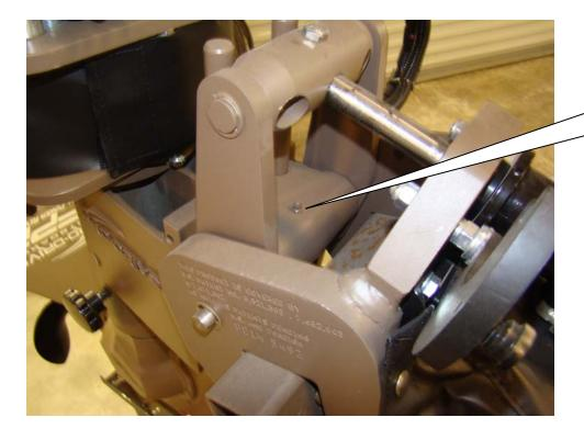
Grease Tower Housing Pivot Pin (15 to 20 Hours)
