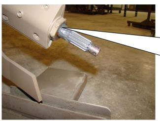
GREASE WILL APPEAR FROM SEAL NUT IN FRONT OF THE PROP WHEN FULL. THIS IS THE AREA WHERE THE DEBRIS IS CLEARED.
