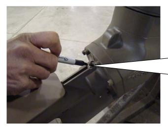
REMOVE ANY GRASS OR FOREIGN DEBRIS FROM THE PROP SHAFT BETWEEN THE PROP AND LOWER UNIT HOUSING. PUMP GREASE INTO THIS GREASE FITTING EVERY 15 to 20 HOURS
