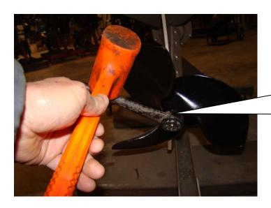
Using a 1-1/8" wrench and a light hammer blow unscrew the nut counter clockwise. Prop can now be slide off spline.
