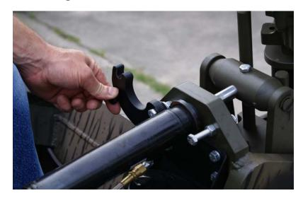
Step 3. Once the unit is in reverse, lock the trim down with the lever loc. \*Note: the reverse lever must not be locked when running in forward gear.
