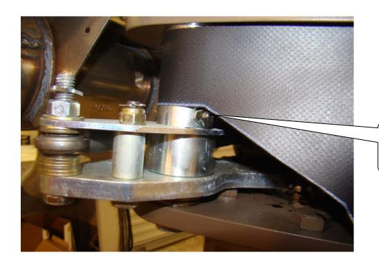
Addition grease fitting for auto reverse. (15 to 20 Hours)
