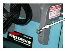
AFTER INSTALLING YOUR MOTOR ON THE BOAT TRANSOM USING THE ALUMINUM SAVER PLATE SUPPLIED WITH THE UNIT, TORQUE THE TRANSOM BOLTS TO 15 FT. LBS. OF TORQUE.
