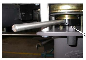
REMOVE THE CLUTCH COVER WRAP AND LOCATE THE HOLE STOP AS SHOWN ON LEFT. INSERT 1/2" BOLT OR PROP PIN INTO THE HOLE STOP. (THE PIN WILL PUSH UP AGAINST THE PLATE POST AS BACK UP WHILE UNSCREWING THE PROP.) \*NOTE: THE PROP UNSCREWS TO THE LEFT.
