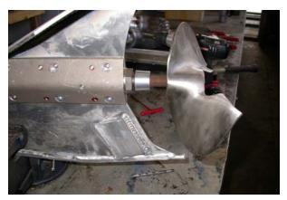
INSTALL THE PROP BY HAND USING GLOVES AND TIGHTEN THOROUGHLY. IT IS NOT NECESSARY TO USE THE WRENCH FOR THIS STEP. ONCE THE PROP IS ON THE SHAFT, REPLACE THE PROP NUT AND TIGHTEN BY USING 1-1/16" WRENCH.
