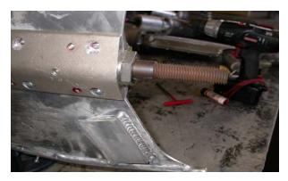
USING LOCKTITE MARINE GRADE ANT-SEIZE OR NEVER SEIZE COAT THE ENTIRE SHAFT.
