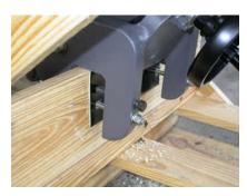
THIS PICTURE OF A UNIT CRATED FOR SHIPMENT SHOWS THE ALL THREAD INSTALLED THROUGH THE TRANSOM SAVER PLATE.
