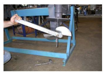
REMOVE PROP NUT USING A 1-1/16" WRENCH OR DEEP WALL SOCKET. NEXT, INSTALL THE PROP WRENCH AS SHOWN. REPLACE NUT TO ENSURE THAT THE PROP WRENCH WILL NOT SLIP OFF WHEN REMOVING PROP. TURN THE WRENCH COUNTER CLOCKWISE UNTIL THE PROP IS REMOVED.
